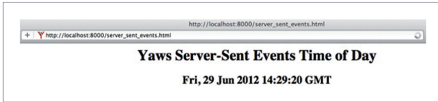
Figure 3. Visiting the server_sent_events example in a browser that supports event streams results in a webpage in which the time of day is dynamically updated once per second.
